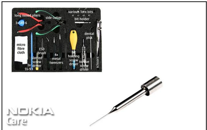
2. You will need the Nokia Standard Toolkit version 2 as well as the hinge opening tool SS-6. Also refer to the General Mechanical Guideline Video for additional hints about the tools and component handling.
