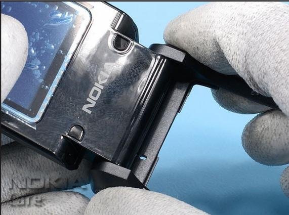
3. Check the mechanical functionality of the Hinge.
