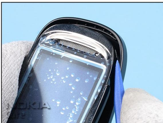
8. Carefully unlock the A-COVER on the top.
