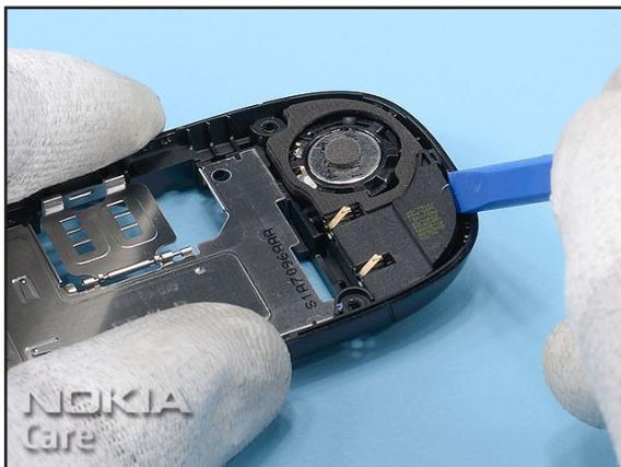
12. Unlock the ANTENNA MODULE with SS-93...
