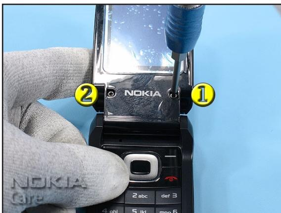
4. Tighten the screws to the torque of 15Ncm in the order shown.
