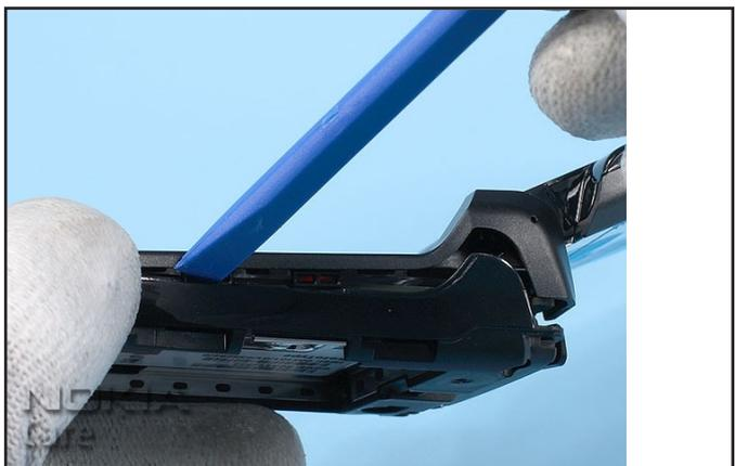
6. Also open the snaps on the left and right side of the Lower Block.
