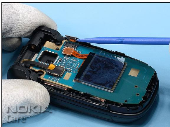
11. Gently open the connector of the LCD PM 128x160 with the SS-93.
