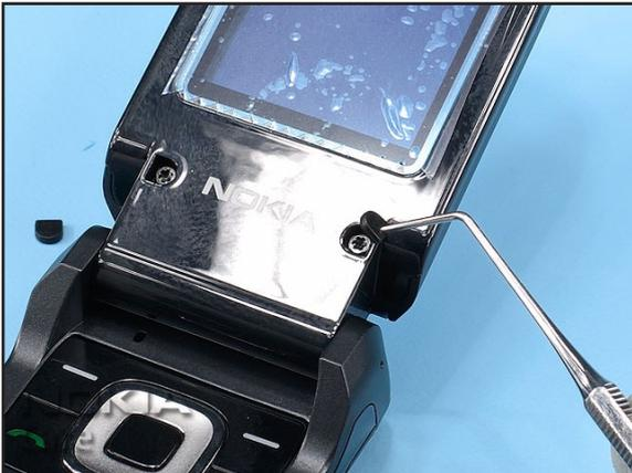
3. Remove the battery if inserted. Cover all sensitive surfaces with the protective film. Remove the SCREW COVER and discard them.
